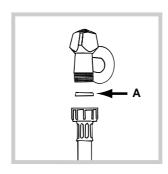
1. Insert seal A into the end of the inlet hose and screw the latter onto a cold water tap with a 3/4 gas threaded opening (see figure). Before performing the connection, allow the water to run freely until it is perfectly clear.
